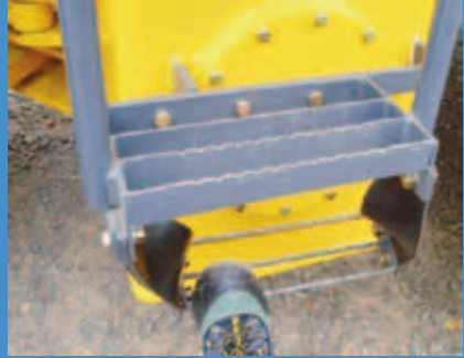
2. This bottom step is too flexible (25kg force should push the step inward by no more than 80mm)
