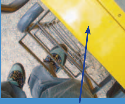
1. This top step has no protection against slipping
